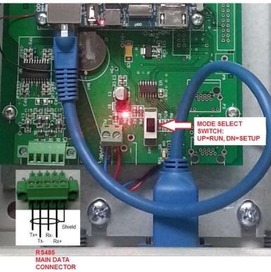
Cable to KCU/KCM/PCM kiln controllers
