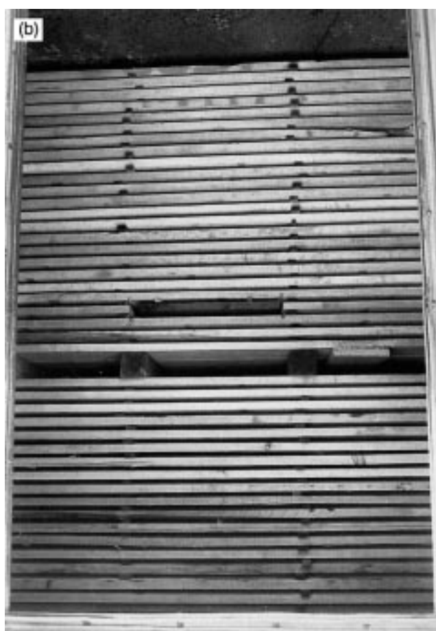
Figure 7.5—Placement of kiln samples in pockets. (a) Schematic of kiln samples placed in pockets built in the side of a load of lumber. Pockets should be deep enough so that the kiln samples do not project beyond the edge of the load. (b) Photograph of kiln sample in place.
