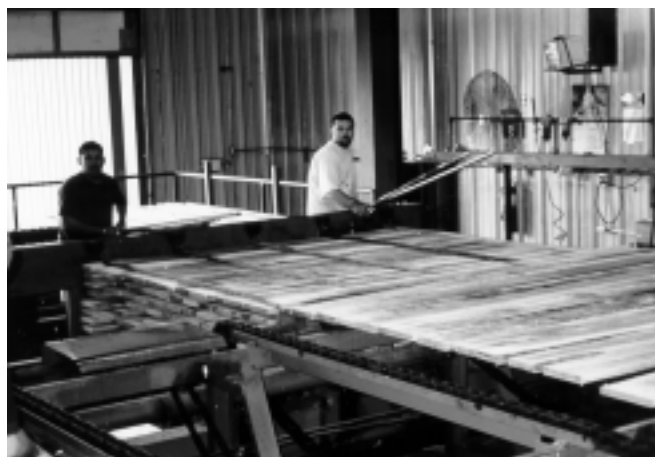
Figure 3.2—Stacking of stickered package of lumber.
